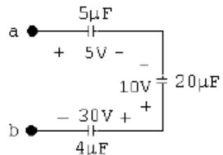
Equivalent capacitance is  $2 \mu\text{F}$  with an initial voltage drop of  $+25 \text{ V}$ .
