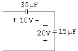
$$\frac{1}{C_3} = \frac{1}{30} + \frac{1}{15} = \frac{1}{10}; \quad C_3 = 10 \mu\text{F}$$
